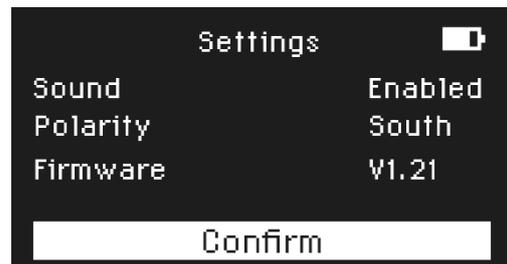
When the Polarity is switched to South, the face of the CELLER8® will be North.
